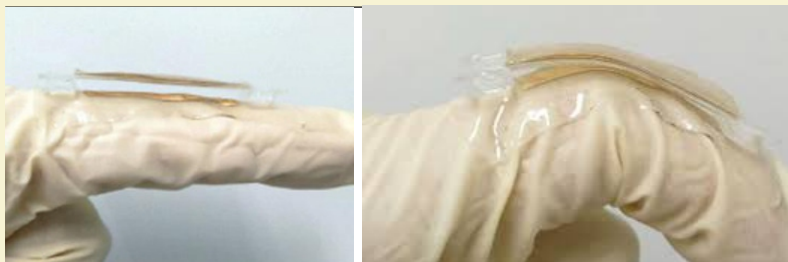
The wearable tab, 1.5cm long by 1cm wide, which lit 48 red LED lights simultaneously
