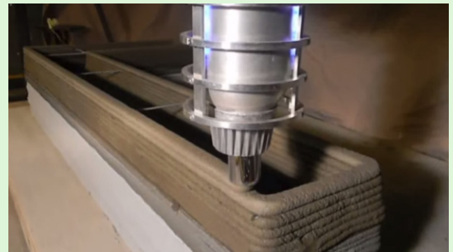
Tip showing laying of concrete layer
